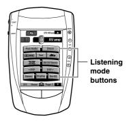
When using the remote controller, select AV Amp in the Home menu to display the operation menu. Then tap the down scroll button to display the next operation menu.
